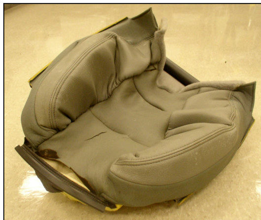
Leather Seat Exposed to Autoclave for 5 hr @121° C
